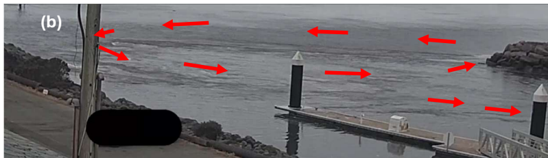
Figure 3. Observation of a transient eddy at the small boat basin entrance. (a) One-minute average surface velocity vector field and overlaid streamlines at 06:19–06:20 PDT on July 30, 2025, demonstrating counter-clockwise shear-driven vortex formation at the entrance. (b) Cropped raw security camera frame at 06:19:37 PDT, visually confirming the surface feature in the raw footage. Arrows denote the direction of fluid motion.
